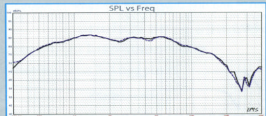
FIGURE 13: EM 1308 two-sample SPL comparison.
